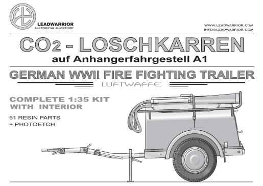
The CO2 Löschgerät auf Anhängerfahrgestell A1 - CO2 fire extinguisher on trailer chassis A1 - was used by the Luftwaffe units to fight fires of the aircrafts, electrical installations, and other devices, were water and foam was not an option.
